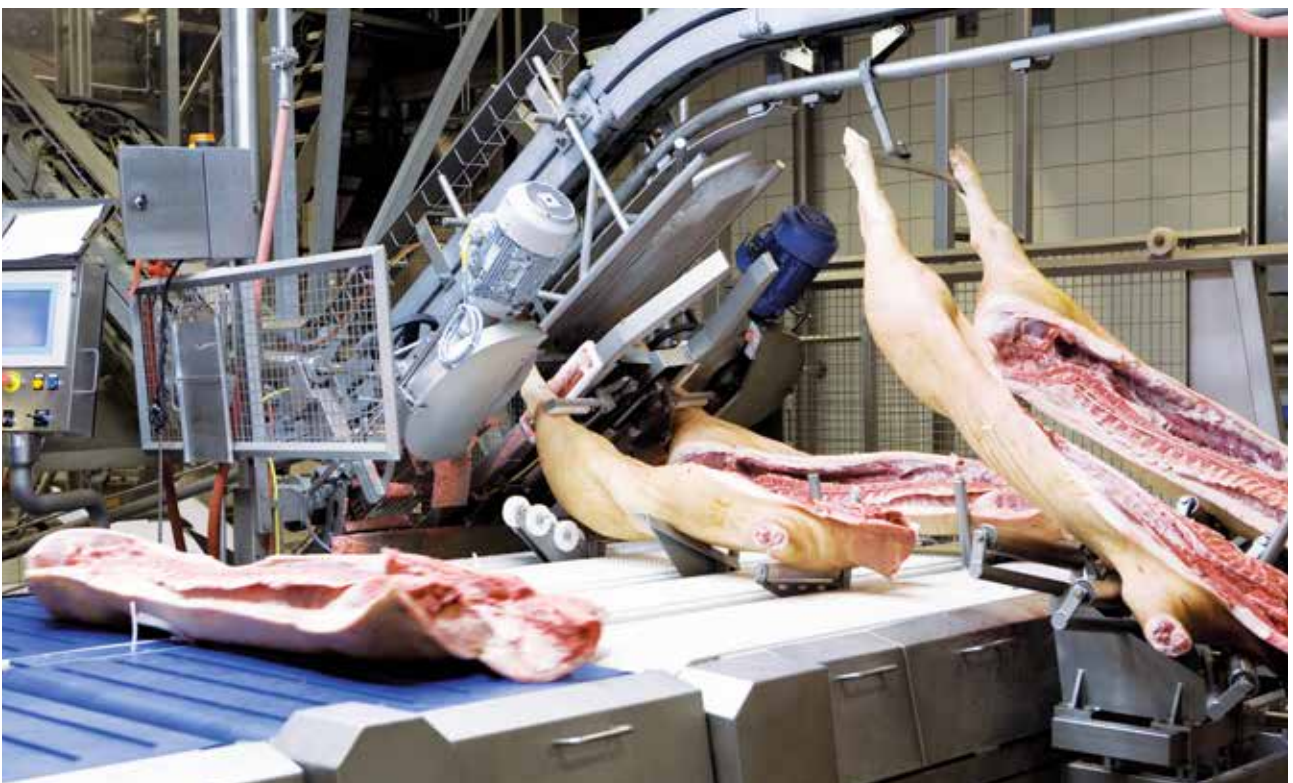
The two half carcasses are automatically lowered onto a conveyor belt, after which the hind toes are sawn off.
