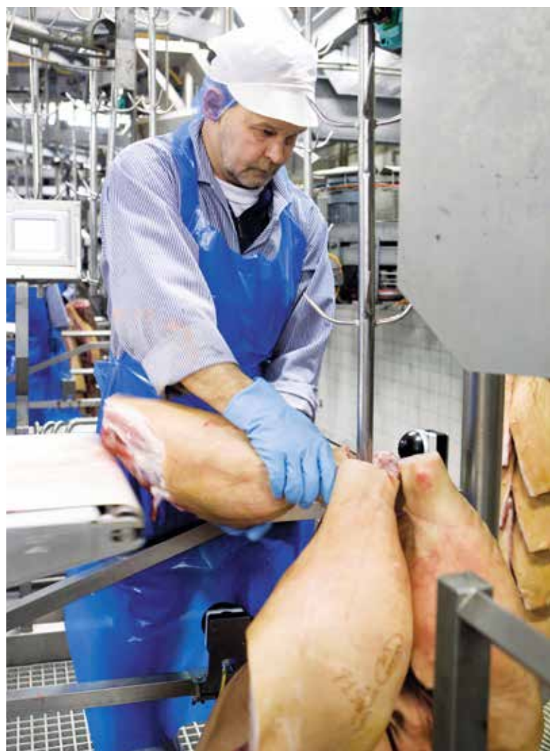
Cuts for further delivery are hung on a 'Christmas tree'. The hanging rails can be adjusted vertically to ensure that the cuts are hung properly.
