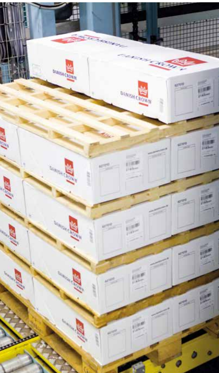
Cartons for freezing are stacked on pallets, at a short interval from one another, to enable rapid and effective freezing down of the meat.
