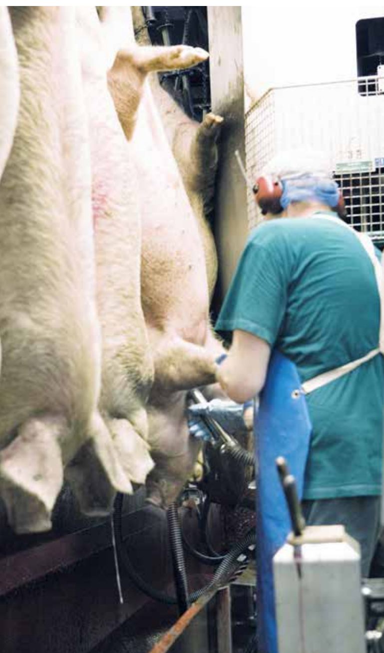
After stunning by CO 2 , sticking and bleeding take place by cutting the carotid arteries without the animal regaining consciousness.
