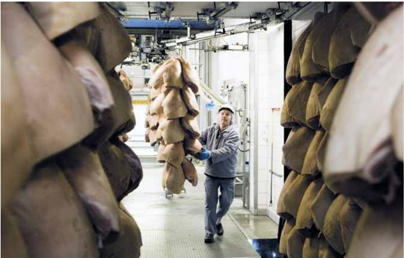
Cuts for further delivery are moved into cold storage or directly onto transport vehicles. The temperature must not exceed 7 °C.
