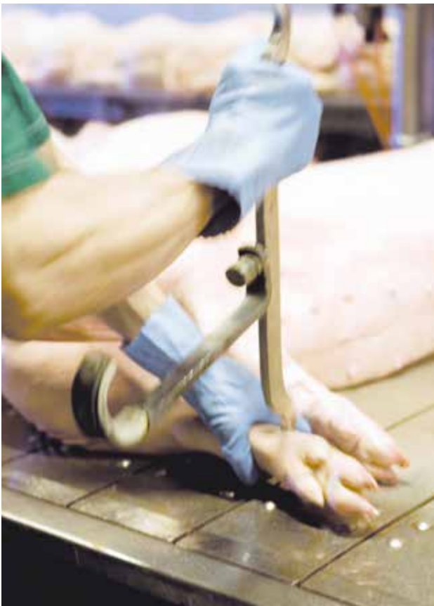
After dehairing, the carcass is hung on a numbered gambrel, which enables its automatic identification during the whole process until cutting.
