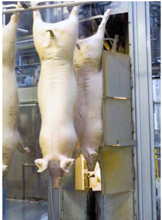
Typically, singeing of the carcass takes place in a furnace at 1000 °C for 6 seconds, thus eliminating bacteria, the remains of bristles and other dirt and preparing the surface of the rind for scraping.
